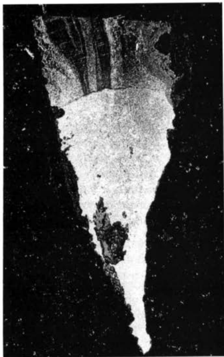
Fig. 630 Knife 4995 showing manufacturing type 2. The edge consists of steel (over-tempered martensite) and contains some dark internal corrosion. Approximately eight layers of ferritic and phosphoric iron make up the back of the knife. The weld appears as a dark line. The weld and several bands in the back are high in arsenic and have all etched in a similar manner. Magnification \times 20
